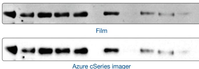
**Figure 1.** The bands on the top are from a chemiluminescent western blot film, scanned. The bottom bands are from the same western blot, taken on an Azure cSeries western imager about one hour later.
