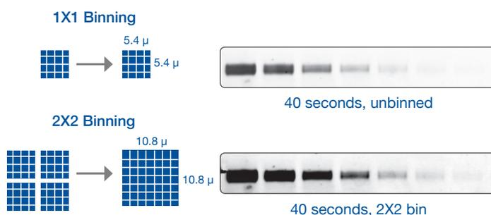
**Figure 2.** Binning is a powerful technique for digital imaging of chemiluminescent western blots. Binning increases sensitivity by combining pixels to make a larger, extra sensitive pixel with a better signal to noise ratio.
