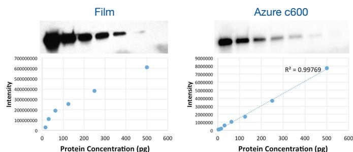
**Figure 5.** An illustration of the difference in linearity between a digital image and x-ray film. For accurate quantitation, signals must be within linear range of each other – the bright signals from the film are saturated and no longer linear. The same blot was imaged on both Lucent Blue X-ray Film and the Azure c600 for 1 minute, and the correlation between the signal and protein concentration is indicated in the two diagrams.
