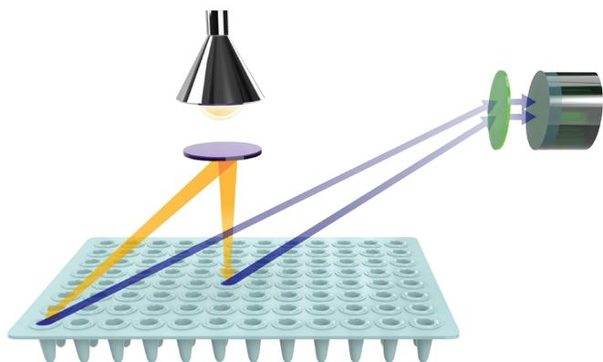
**Figure 1. Schematic representation of whole plate imaging using a conventional Real-Time PCR system.** The well in the center of the block has a shorter light path (yellow) and therefore emits a higher fluorescence signal compared to the well at the corner (blue), which has a longer light path.
